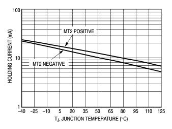
Figure 3. Typical Holding Current versus Junction Temperature
