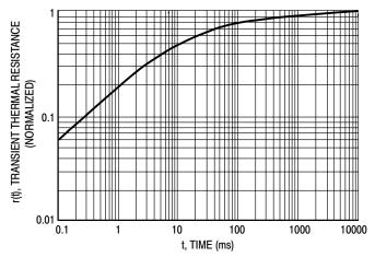
Figure 8. Typical Thermal Response
