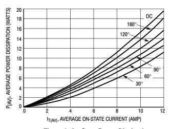
Figure 6. On-State Power Dissipation
