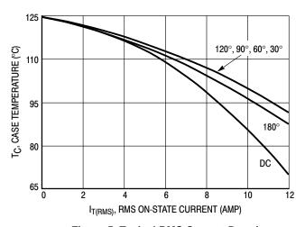
Figure 5. Typical RMS Current Derating
