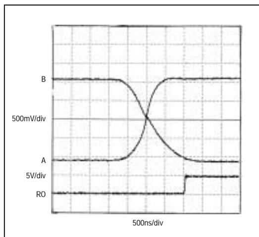
Figure 12. Receiver  $t_{PLH}$
