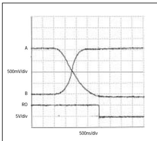
Figure 11. Receiver  $t_{PHL}$
