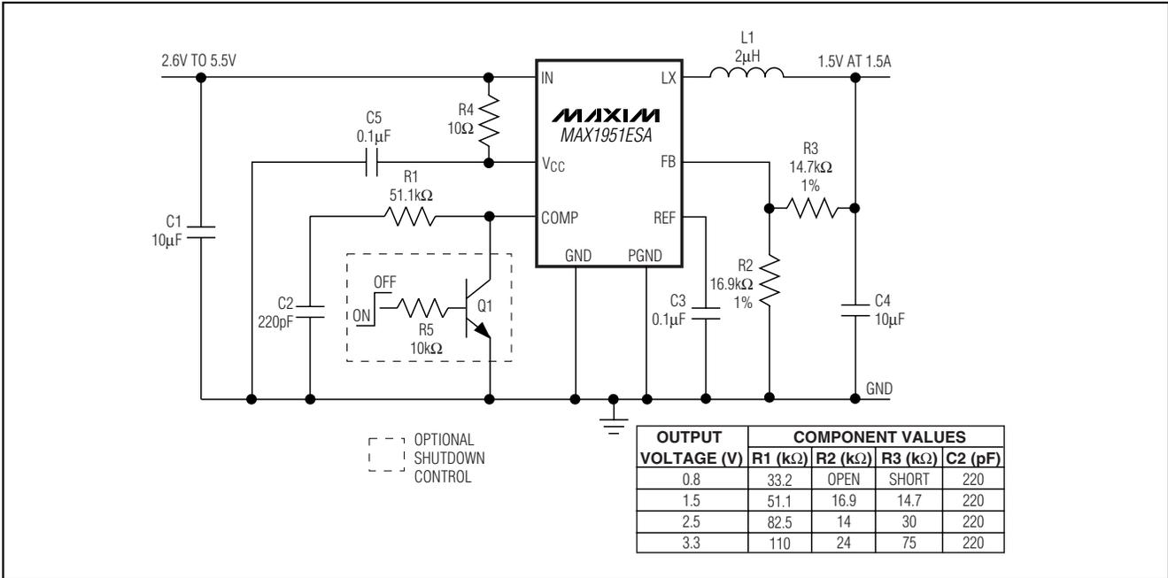
Figure 2a. MAX1951 Adjustable Output Typical Application Circuit
