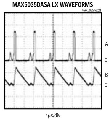
A: SWITCH VOLTAGE (LX PIN), 20V/div ( $V_{IN} = 48V$ )
