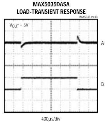
A:  $V_{OUT}$ , 200mV/div, AC-COUPLED
