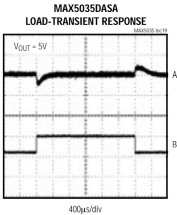
A:  $V_{OUT}$ , 200mV/div, AC-COUPLED
