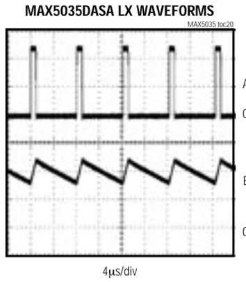
A: SWITCH VOLTAGE (LX PIN), 20V/div ( $V_{IN} = 48V$ )
