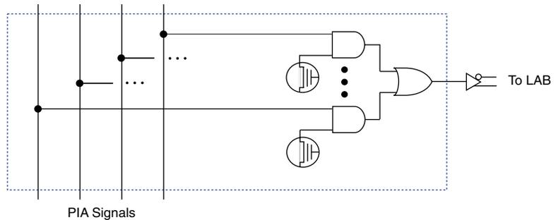
While the routing delays of channel-based routing schemes in masked or FPGAs are cumulative, variable, and path-dependent, the MAX 7000 PIA has a fixed delay. The PIA thus eliminates skew between signals and makes timing performance easy to predict.
