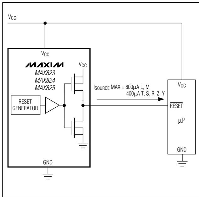
Figure 4. Interfacing to  $\mu$ Ps with Bidirectional Resets
