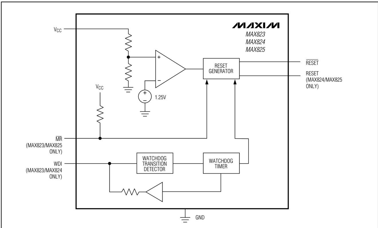
Figure 1. Functional Diagram
