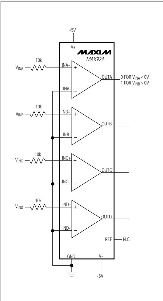
Figure 8. Level Shifter: ±5V Input to CMOS Output
