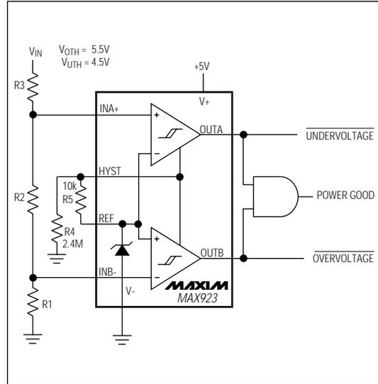
Figure 6. Window Detector
