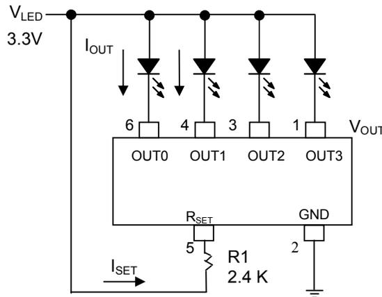
※Neither an inductor, a capacitor nor Schottky diode is needed.
