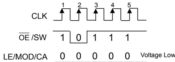
The above signal sequence example can make MBI5368 resume to the Normal Mode.
