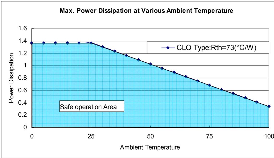
The maximum allowable package power dissipation is determined as  $P_D(max) = (T_j - T_a) / R_{th(j-a)}$ . When 24 output channels are turned on simultaneously, the actual package power dissipation is  $P_D(act) = (I_{DD} \times V_{DD}) + (I_{OUT} \times Duty \times V_{DS} \times 24)$ . Therefore, to keep  $P_D(act) \leq P_D(max)$ , the allowable maximum output current as a function of duty cycle is:
