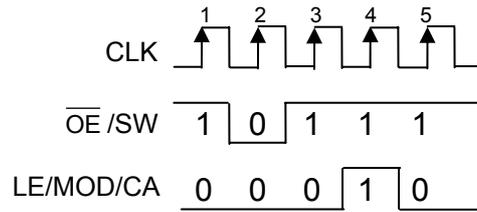
The above shows an example of the signal sequence that can set the next operation mode of MBI5368 to be the Current Adjust Mode. The LE/MOD/CA active pulse here would not latch any serial data.
