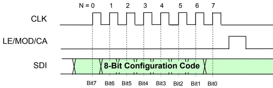
In the Current Adjust Mode, by sending the positive pulse of LE/MOD/CA, the content of the Shift Register with a Configuration Code will be written to the 8-bit Configuration Latch.
