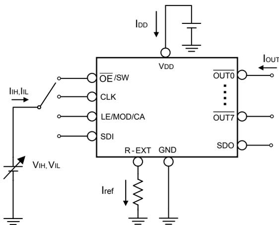
**Test Circuit for Switching Characteristics**
