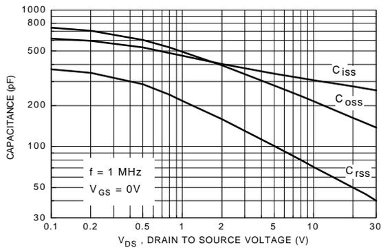
**Figure 9. Capacitance Characteristics**
