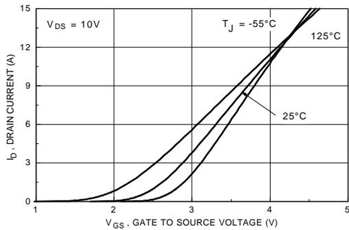
Figure 5. Transfer Characteristics
