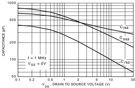
**Figure 9. Capacitance Characteristics**
