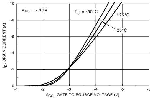
Figure 5. Transfer Characteristics
