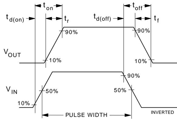
**Figure 12. Switching Waveforms**
