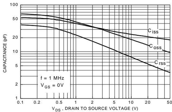
**Figure 9. Capacitance Characteristics.**
