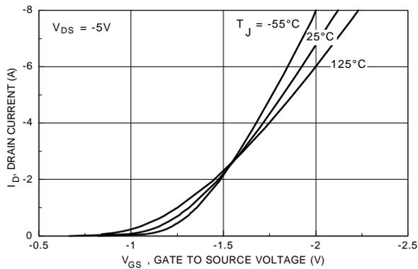
Figure 5. Transfer Characteristics.
