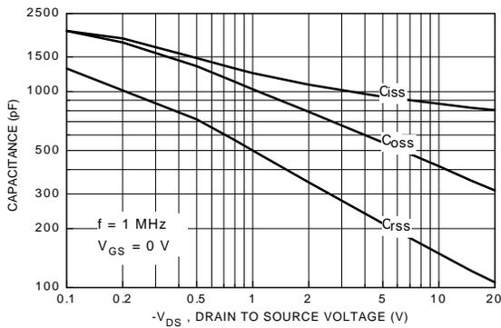
**Figure 9. Capacitance Characteristics.**
