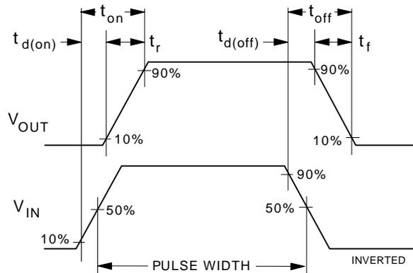
**Figure 12. Switching Waveforms.**
