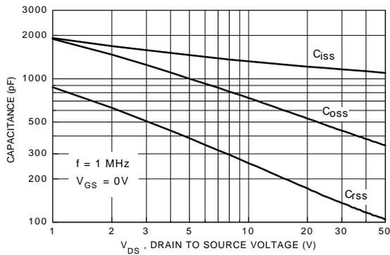
**Figure 9. Capacitance Characteristics**
