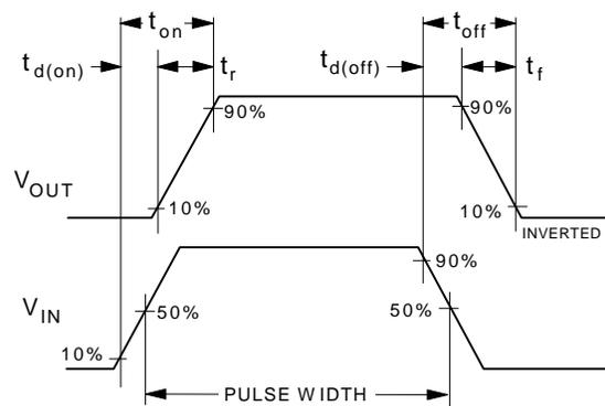
**Figure 12. Switching Waveforms**
