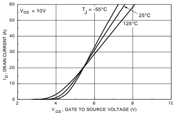
Figure 5. Transfer Characteristics
