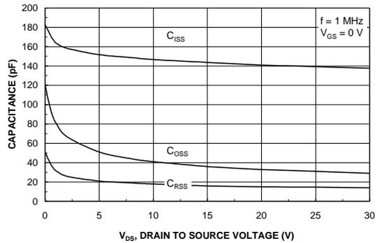
Figure 8. Capacitance Characteristics.
