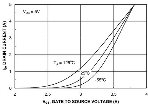
Figure 5. Transfer Characteristics.
