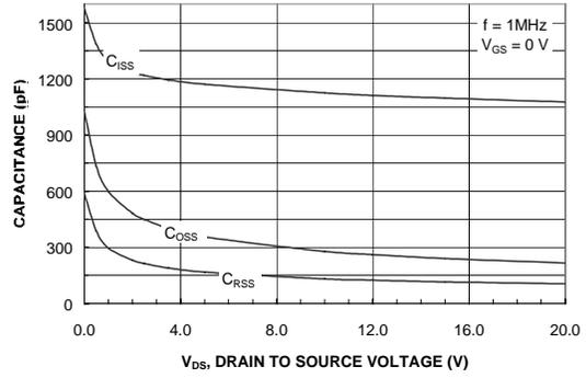
Figure 8. Capacitance Characteristics.
