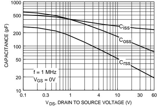
Figure 8. Capacitance Characteristics.
