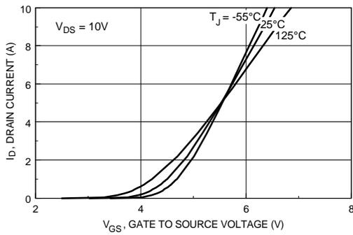
Figure 5. Transfer Characteristics.
