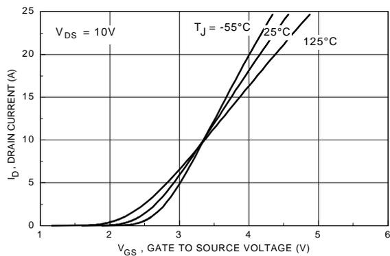
Figure 5. Transfer Characteristics.
