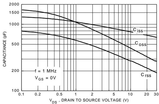
**Figure 9. Capacitance Characteristics.**
