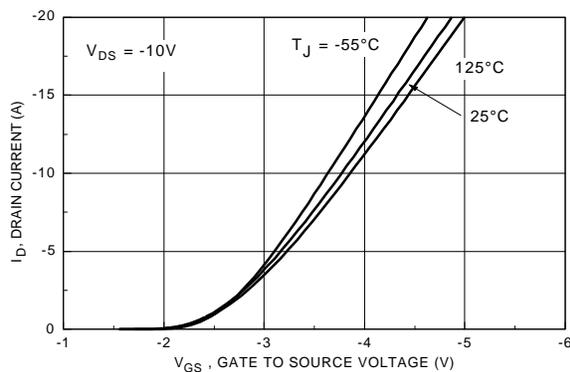
Figure 5. Transfer Characteristics.
