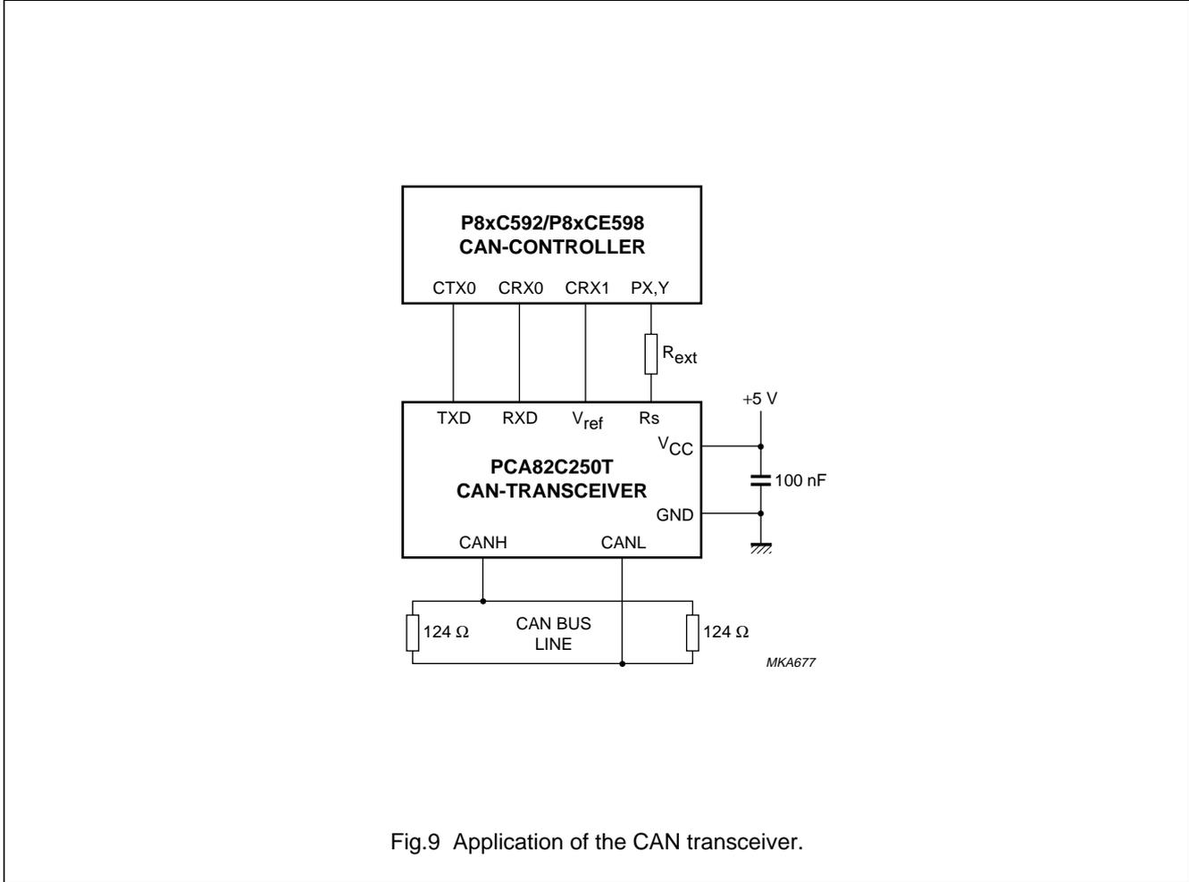
Fig.9 Application of the CAN transceiver.
