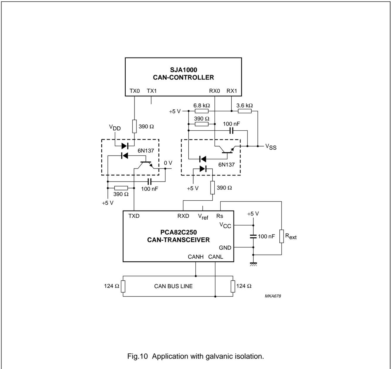
Fig.10 Application with galvanic isolation.
