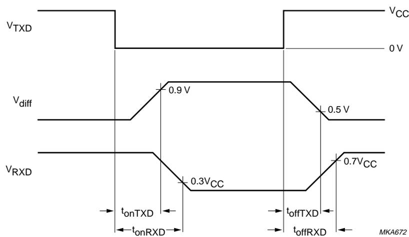
Fig.4 Timing diagram for dynamic characteristics.
