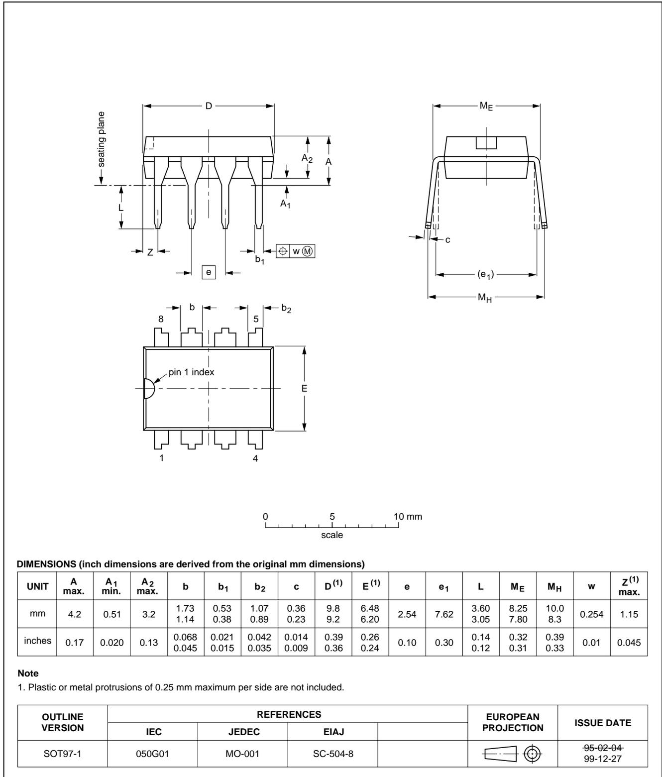
DIMENSIONS (inch dimensions are derived from the original mm dimensions)
