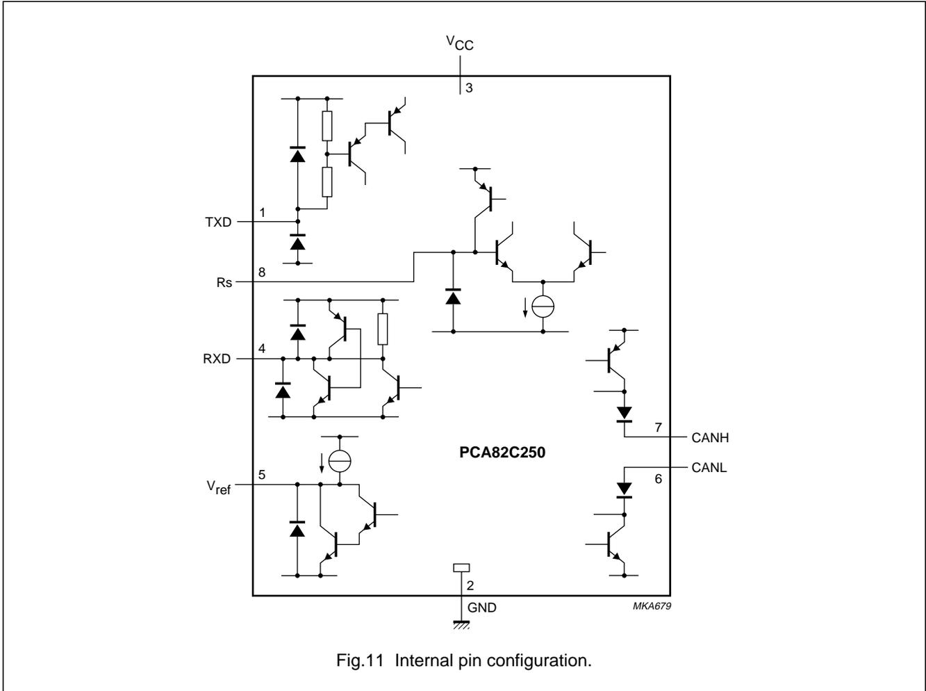
Fig.11 Internal pin configuration.
