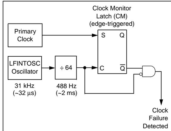
The FSCM function is enabled by setting the FCMEN bit in the Configuration Word register (CONFIG). It is applicable to all external clock options (LP, XT, HS, EC, RC or IO modes).
