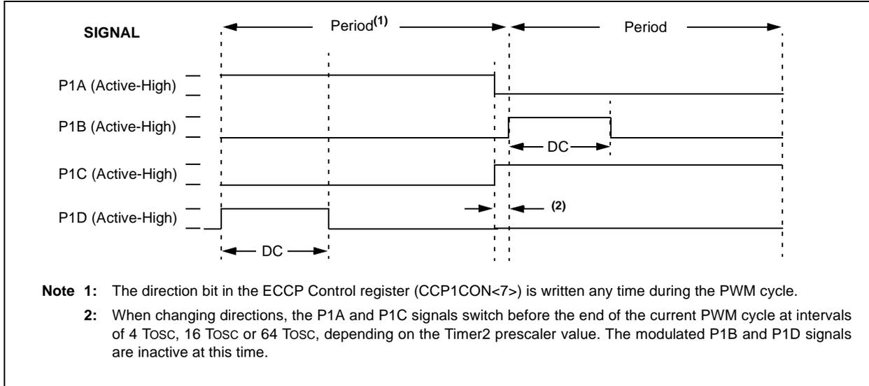
**FIGURE 11-11: PWM DIRECTION CHANGE AT NEAR 100% DUTY CYCLE**
