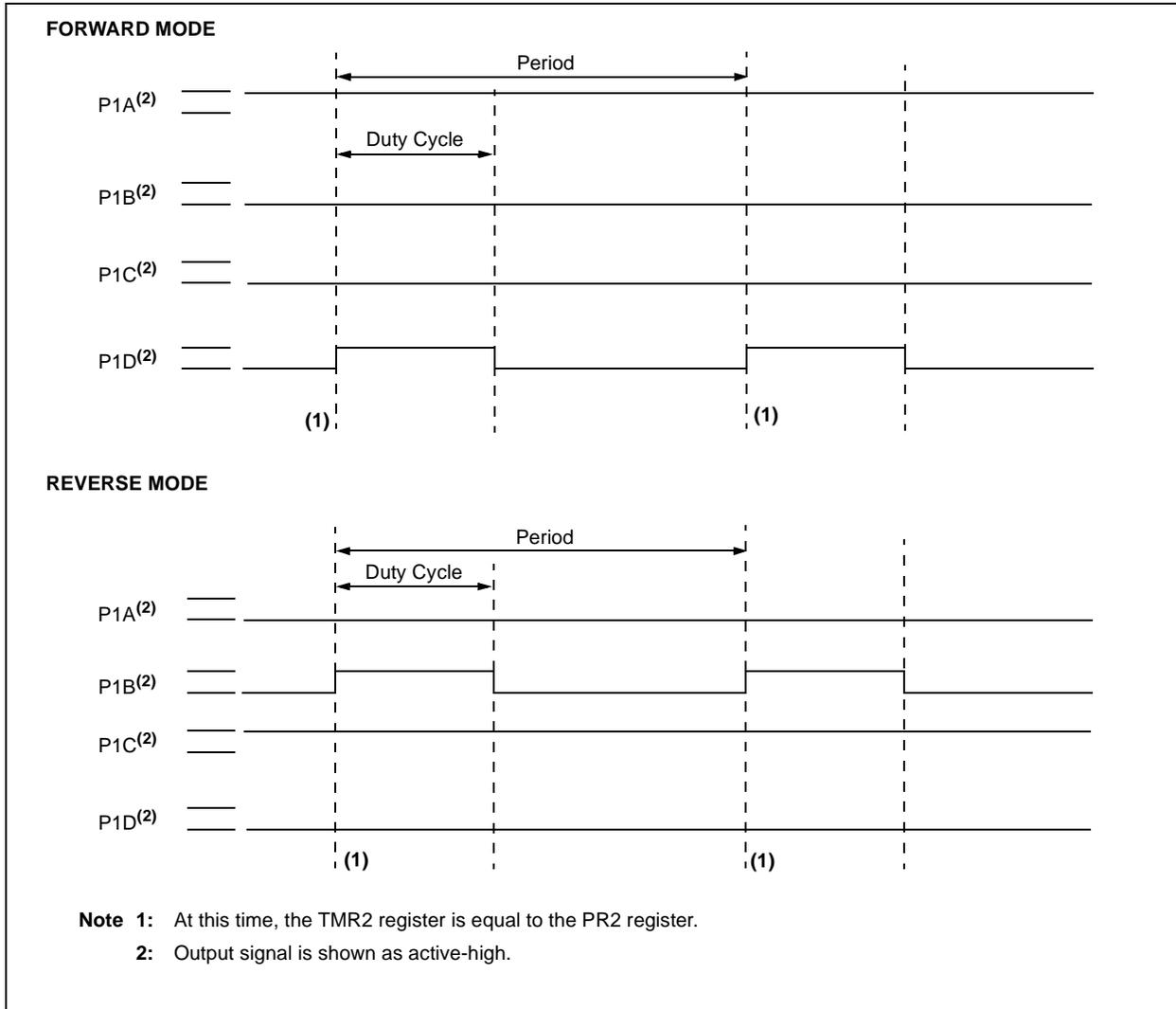
**FIGURE 11-9: EXAMPLE OF FULL-BRIDGE APPLICATION**
