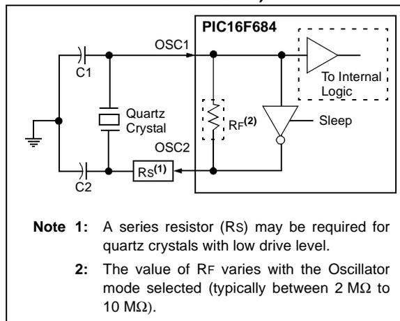
**Note 1:** Quartz crystal characteristics vary according to type, package and manufacturer. The user should consult the manufacturer data sheets for specifications and recommended application.
