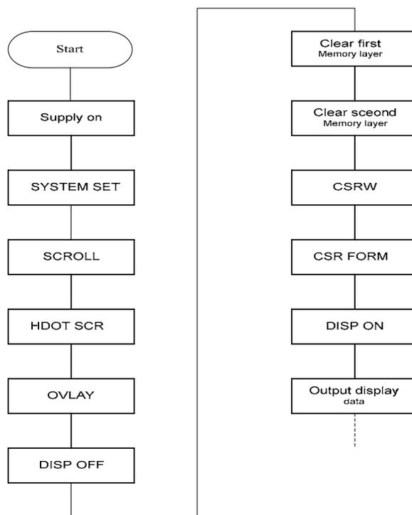
**Figure 8-1: Initialization Procedure**
