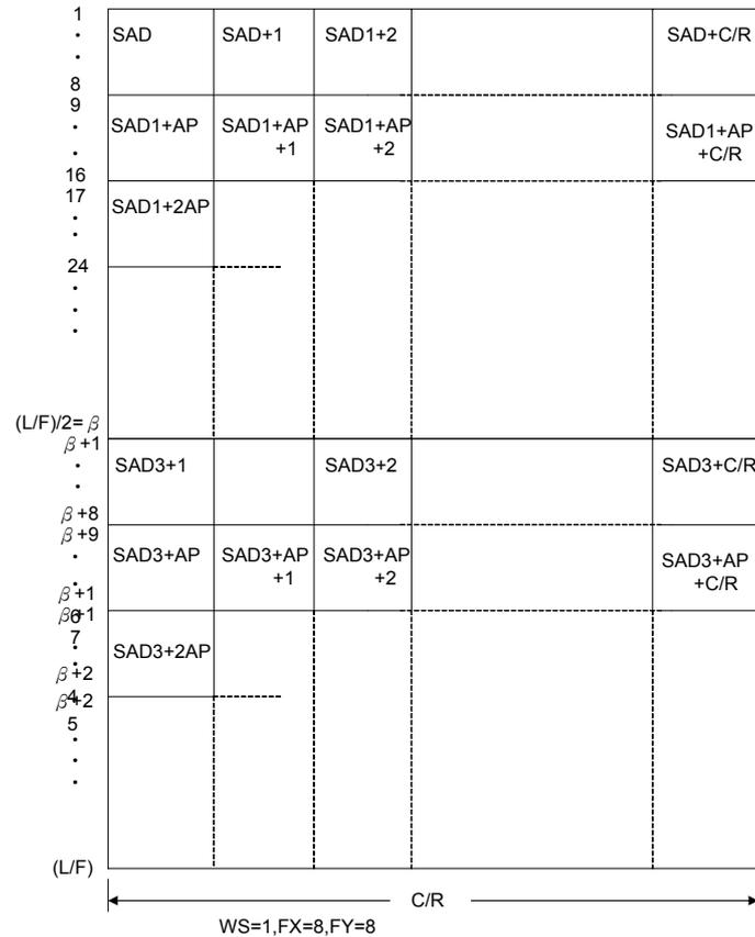
**Figure 7-14: Two-panel Display Address Indexing**
