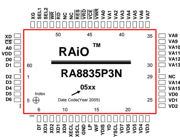
Figure 4-1: RA8835P3N(QFP-60 Pin)
