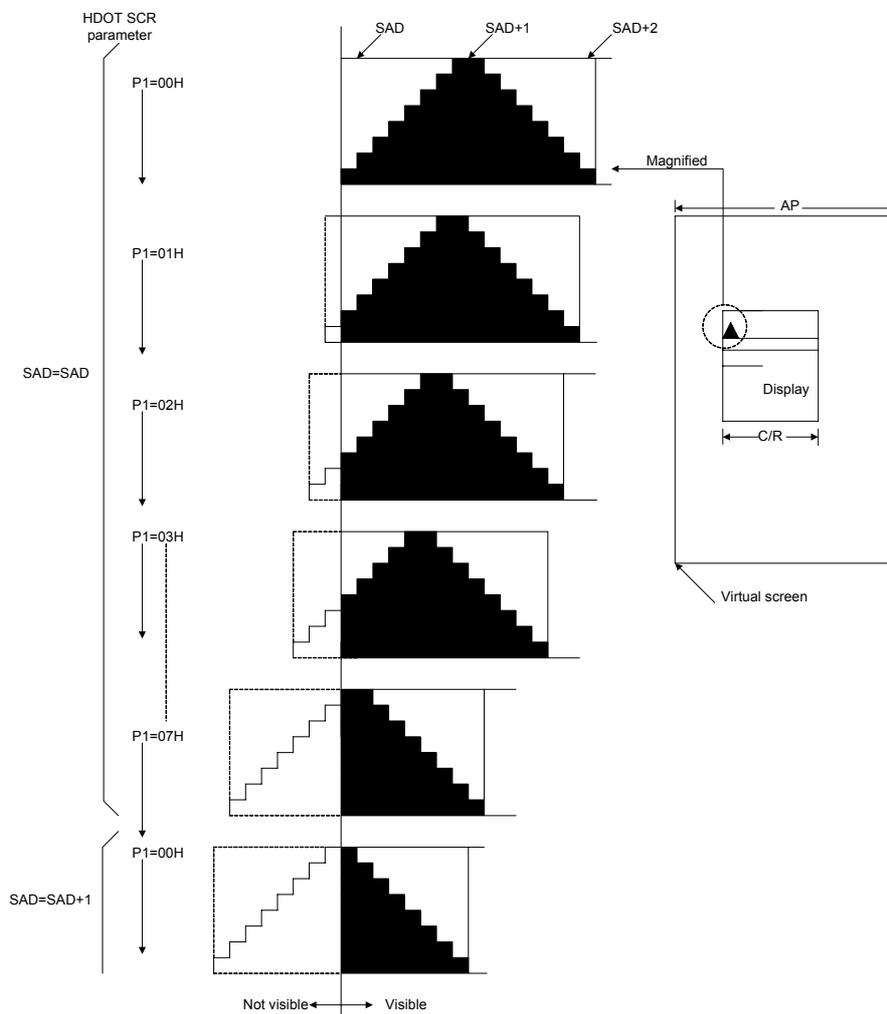
**Figure: 8-7 HDOT SCR Example**
