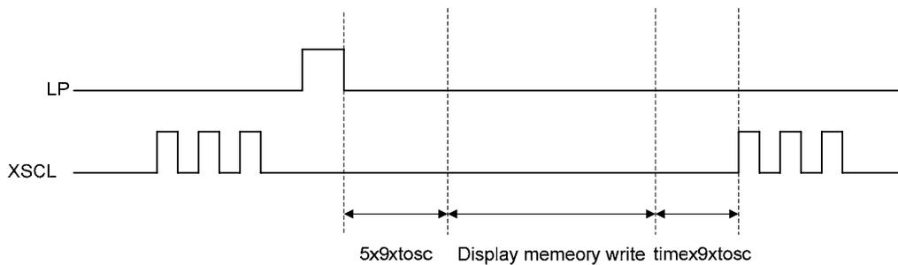
The allowable writing duration is since “5 x 9 x t<sub>osc</sub>” has elapsed (t<sub>osc</sub> = 1/f<sub>osc</sub>: a cycle of the oscillation frequency) from the positive going edge of LP up to {(TCR) – (C/R) – 7} x 9 x t<sub>osc</sub>.
