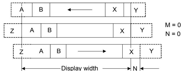
M/N is the number of bits(dots) that parameter 1 (P1) is incremented/decremented by.
