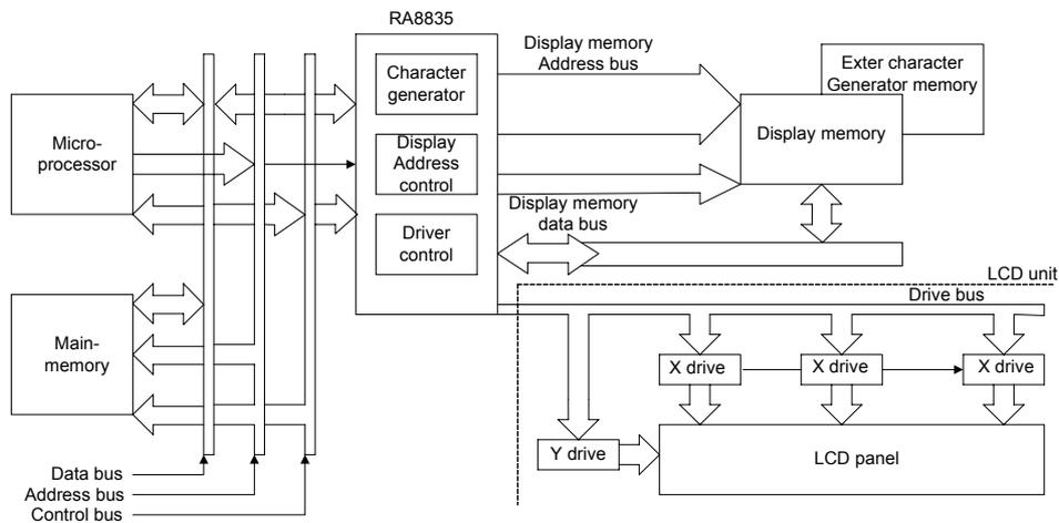
**Figure 8-5: System Block Diagram**
