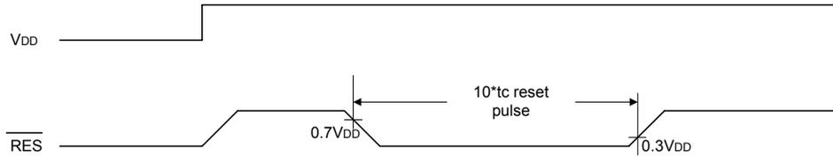
**Figure 7-8: Reset Timing**
