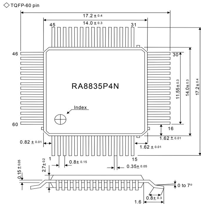
Note: Both of the RA8835P3N and RA8835P4N are use “lead-free” package for ROHS compliance.
