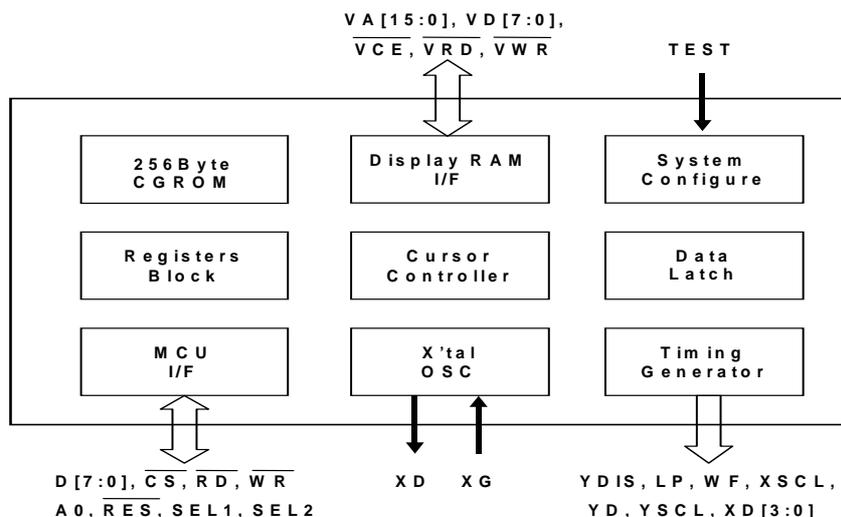
Figure 3-1: Block Diagram
