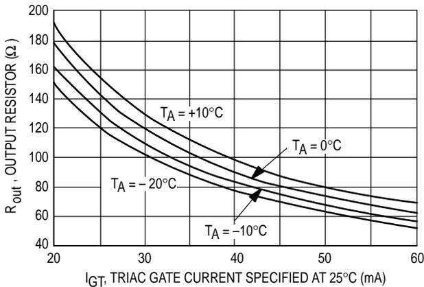
**Figure 5. Minimum Output Current versus Output Resistor**
