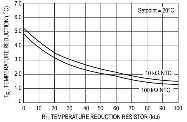
**Figure 14. Temperature Reduction versus Temperature Setpoint**
