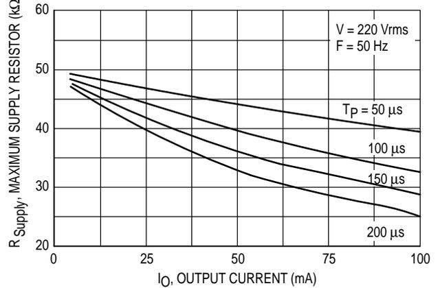
**Figure 10. Maximum Supply Resistor versus Output Current**
