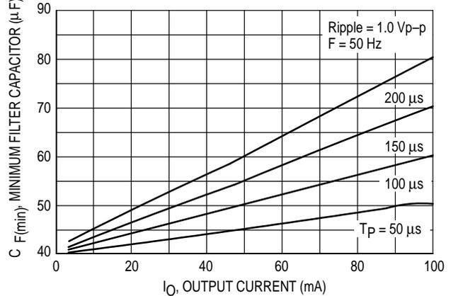
**Figure 12. Minimum Filter Capacitor versus Output Current**
