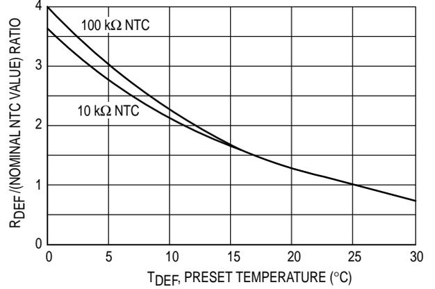
**Figure 16.  $R_S + R_2$  versus Preset Setpoint**
