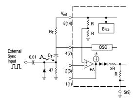
The diode clamp is required if the Sync amplitude is large enough to cause the bottom side of CT to go more than 300 mV below ground.
