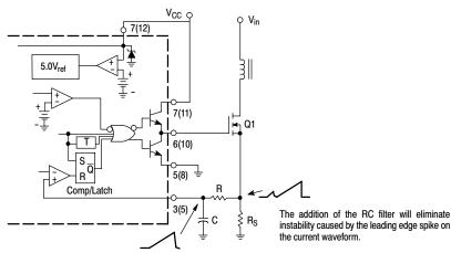
Figure 24. Current Waveform Spike Suppression
