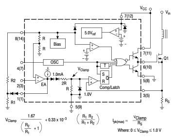
Figure 20. Adjustable Reduction of Clamp Level
