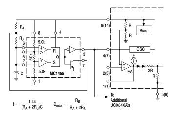
Figure 19. External Duty Cycle Clamp and Multi–Unit Synchronization
