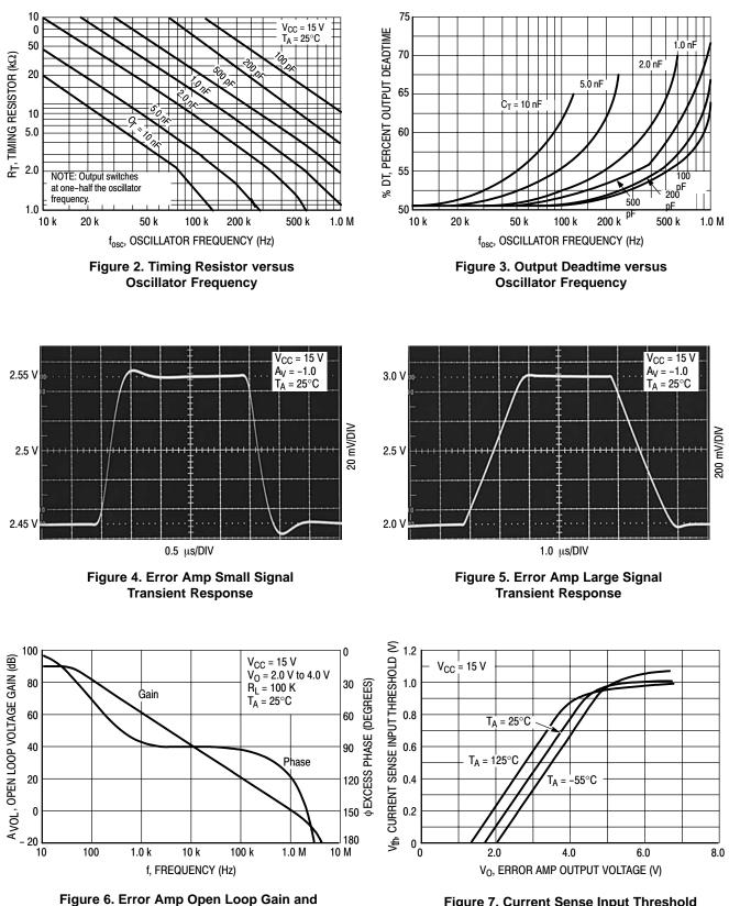
Figure 7. Current Sense Input Threshold versus Error Amp Output Voltage
