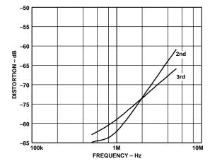
Figure 14. Harmonic Distortion vs. Frequency
