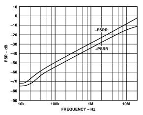
Figure 10. Power Supply Rejection vs. Frequency
