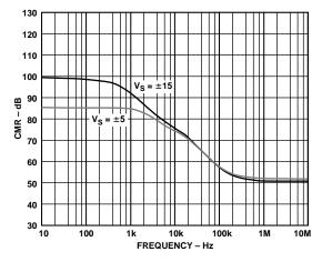
Figure 11. Common-Mode Rejection vs. Frequency
