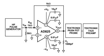
Figure 23. Inverting Amplifier Connection
