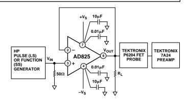
Figure 18. Noninverting Amplifier Connection
