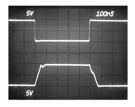
Figure 24. Inverting Large Signal Pulse Response,  $R_L = 1 \ \mathrm{k}\Omega$
