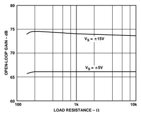
Figure 9. Open-Loop Gain vs. Load Resistance
