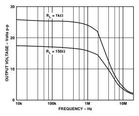
Figure 12. Large Signal Frequency Response; G = +2
