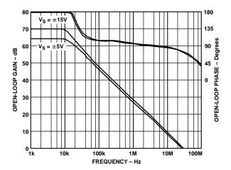
Figure 8. Open-Loop Gain and Phase Margin vs. Frequency
