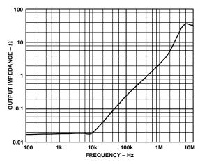
Figure 6. Closed-Loop Output Impedance vs. Frequency
