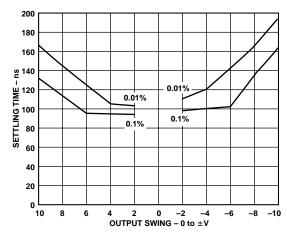
Figure 13. Output Swing and Error vs. Settling Time
