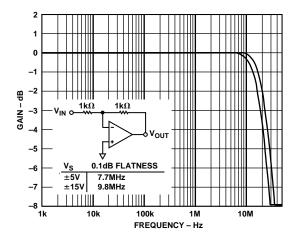
Figure 17. Closed-Loop Gain vs. Frequency, Gain = -1
