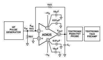
Figure 26a. Inverting Amplifier Driving a Capacitive Load
