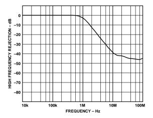
Figure 29. Frequency Response of Second Order Butterworth Filter
