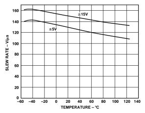
Figure 15. Slew Rate vs. Temperature
