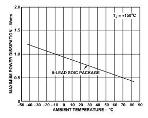
Figure 2. Maximum Power Dissipation vs. Temperature
