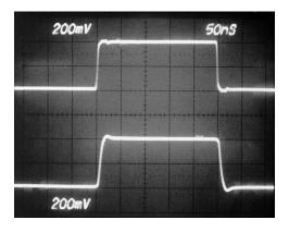
Figure 20. Noninverting Small Signal Pulse Response,  $R_L=1~\mathrm{k}\Omega$
