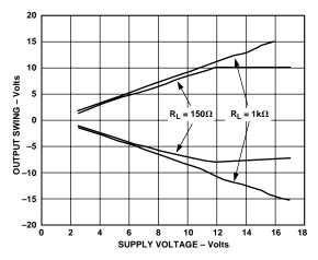
Figure 3. Output Voltage Swing vs. Supply
