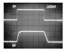
Figure 19. Noninverting Large Signal Pulse Response,  $R_{\rm L}$  = 1  $k\Omega$
