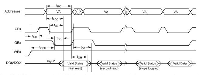
**Note:** VA = Valid address; not required for DQ6. Illustration shows first two status cycle after command sequence, last status read cycle, and array data read cycle.
