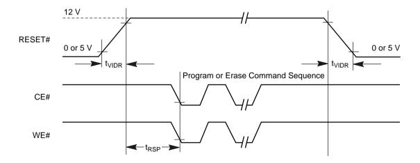
Figure 11. Temporary Sector Unprotect Timing Diagram (Am29F002B only)
