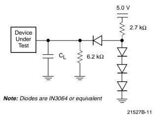
Figure 3. Test Setup
