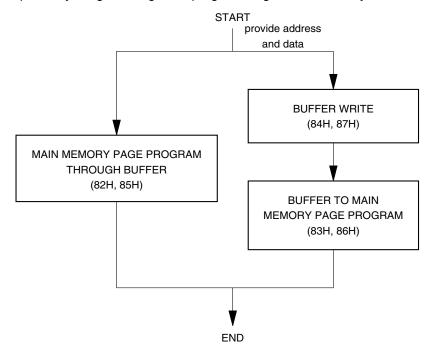
Notes: 1. This type of algorithm is used for applications in which the entire array is programmed sequentially, filling the array page-by-page.
