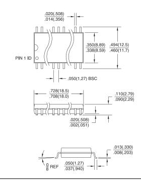
**8S2**, 8-lead, 0.210" Wide, Plastic Gull Wing Small Outline (EIAJ SOIC) Dimensions in Inches and (Millimeters)
