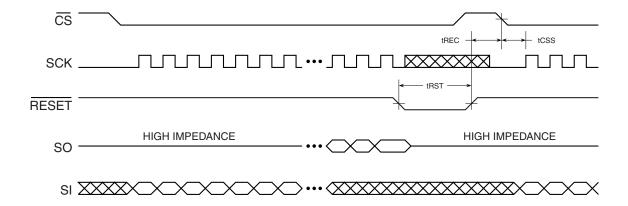
Note: The  $\overline{\text{CS}}$  signal should be in the high state before the  $\overline{\text{RESET}}$  signal is deasserted.
