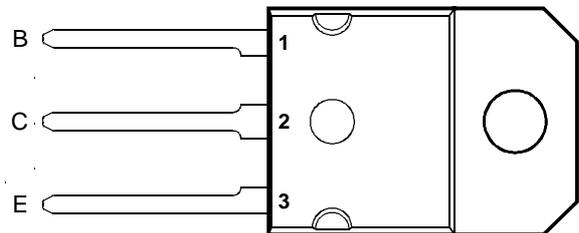
Pin 2 is in electrical contact with the mounting base.
