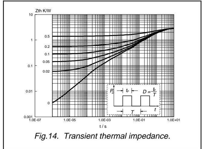
Silicon Diffused Power Transistor
