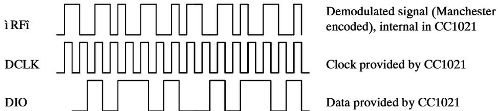
**Figure 10. Synchronous Manchester encoded mode ( $SEP\_DI\_DO = 0$ )**
