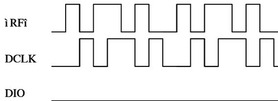
Demodulated signal (NRZ), internal in CC1021
