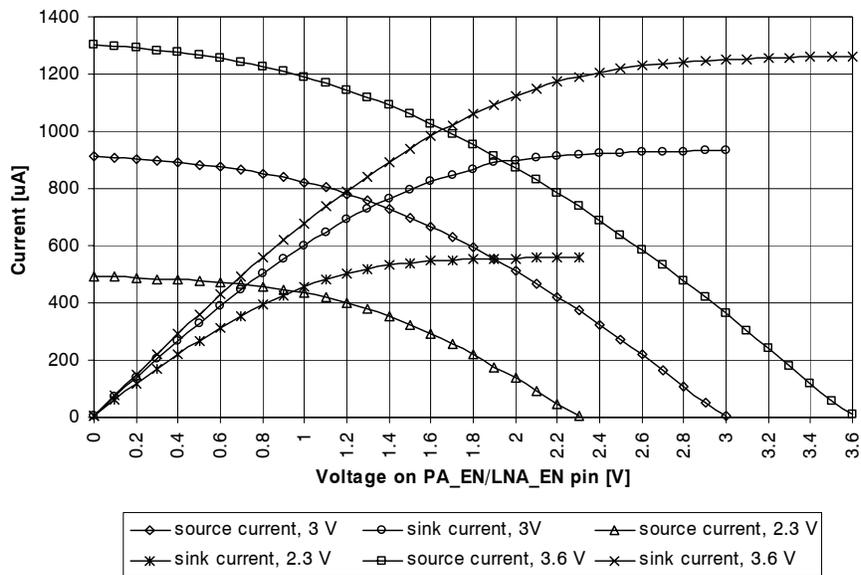
Figure 35. PA\_EN and LNA\_EN pin drive
