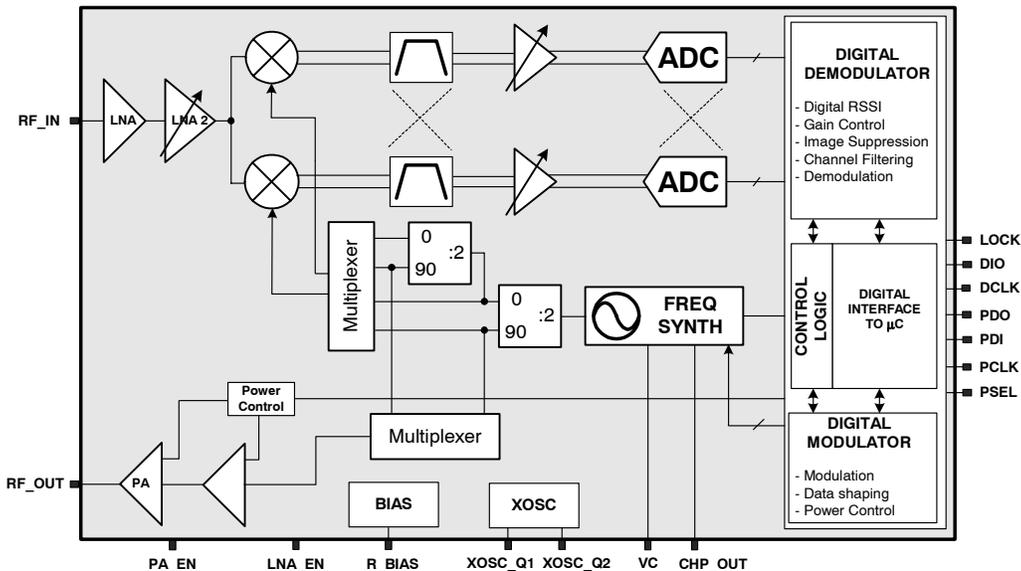
Figure 2. **CC1021** simplified block diagram
