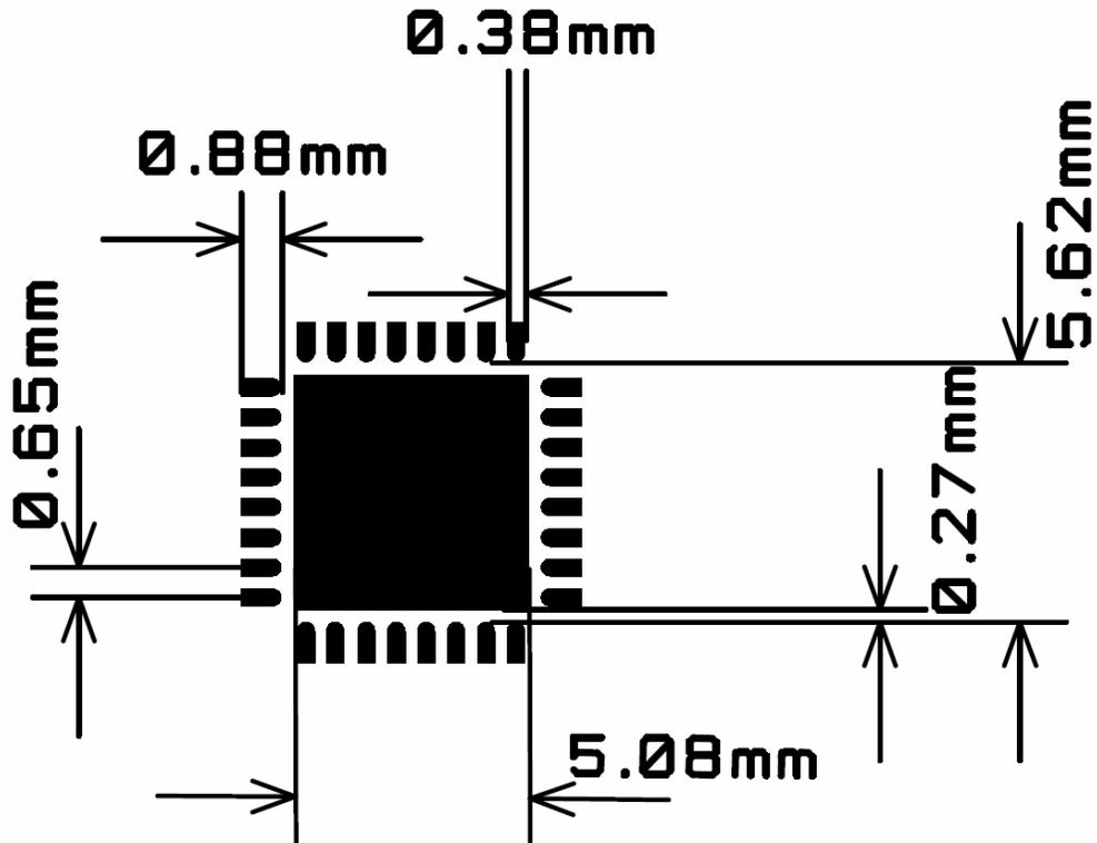
**Note:** The figure is an illustration only and not to scale. There are nine 14 mil (0.36 mm) diameter via holes distributed symmetrically in the ground plane under the package. See also the CC1020EMX reference design.
