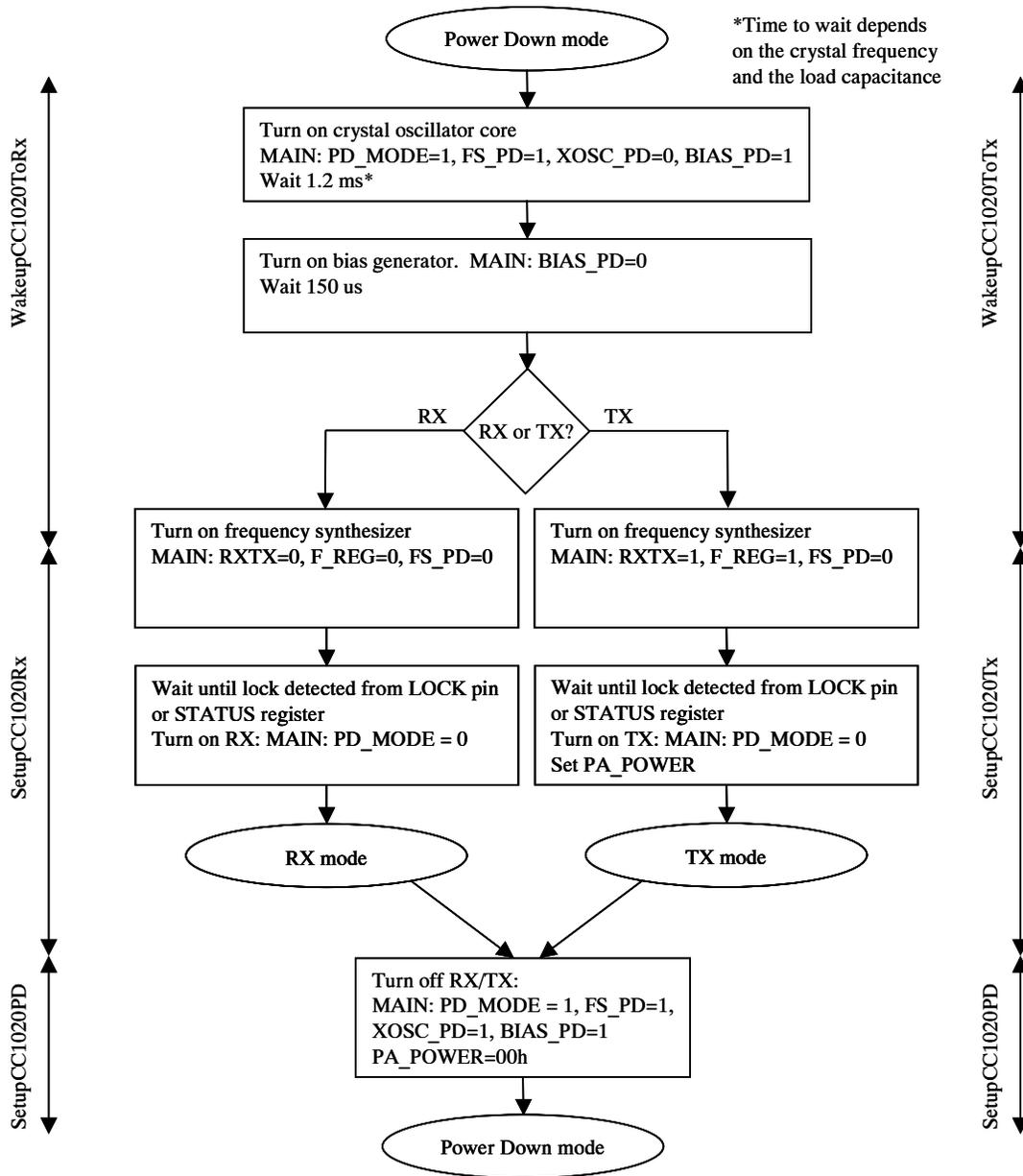
Figure 31. Sequence for activating RX or TX mode
