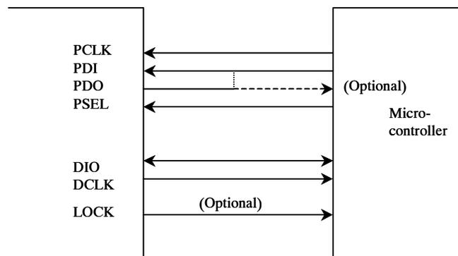
Figure 6. Microcontroller interface
