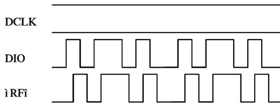
DCLK is not used in transmit mode, and is used as data output in receive mode. It can be set to default high or low in transmit mode.
