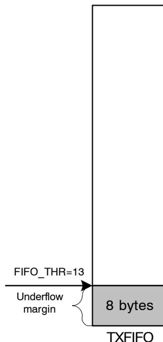
**Figure 13: Example of FIFO at threshold**
