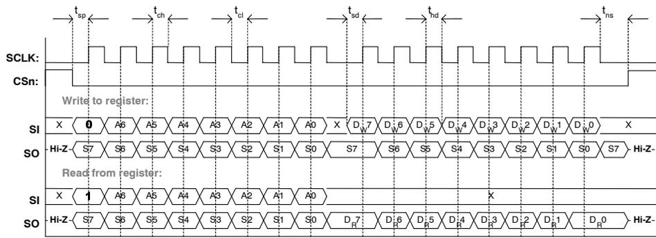
Figure 6: Configuration registers write and read operations
