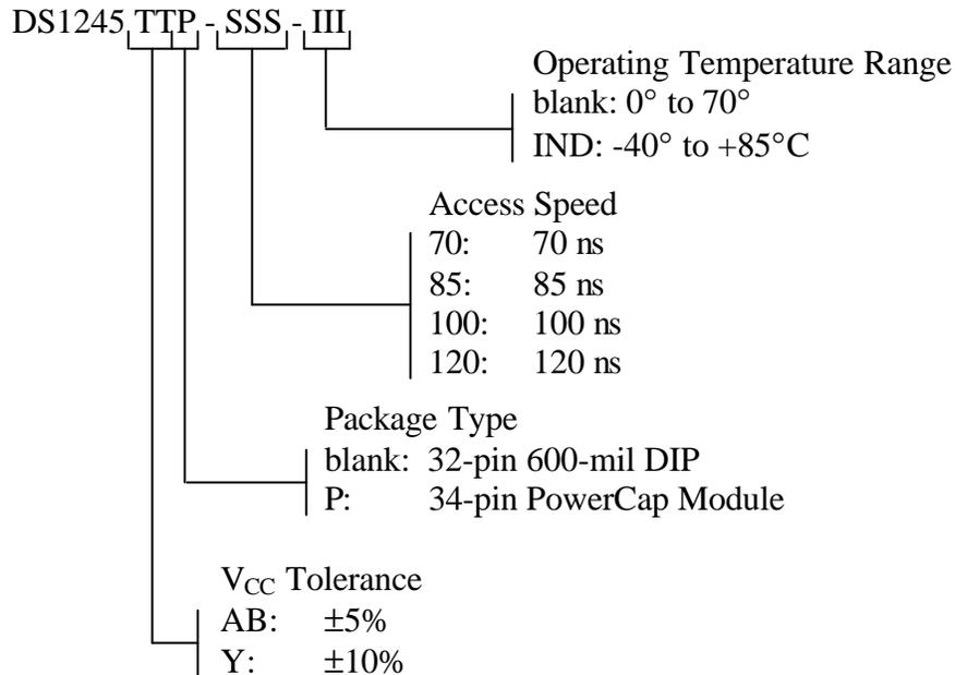
**DS1245Y/AB NONVOLATILE SRAM, 32-PIN, 740-MIL EXTENDED DIP MODULE**
