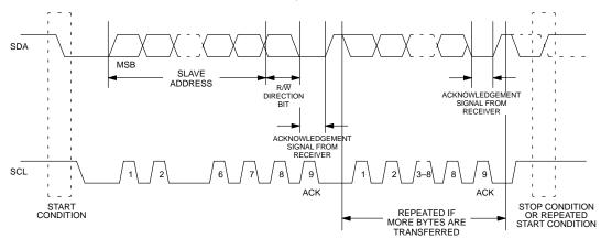
Figure 4 details how data transfer is accomplished on the two–wire bus. Depending upon the state of the  $R/\overline{W}$  bit, two types of data transfer are possible:
