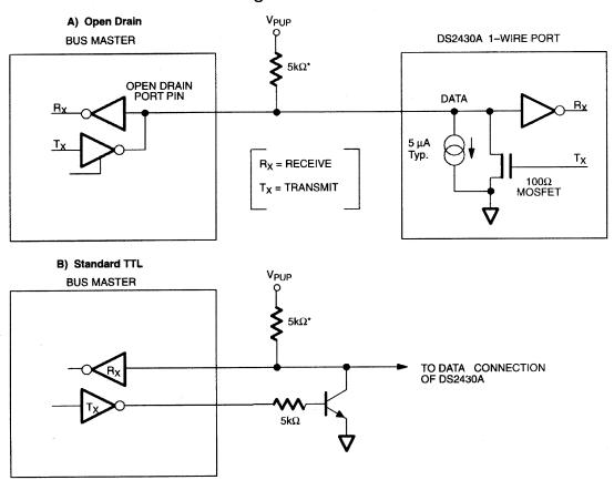
\*5 k $\Omega$  is adequate for reading the DS2430A. To write to a single device, a 2.2 k $\Omega$  resistor and V<sub>PUP</sub> of at least 4.0V is sufficient. For writing multiple DS2430As simultaneously or operation at low V<sub>PUP</sub>, the resistor should be bypassed by a low-impedance pullup to V<sub>PUP</sub> while the device copies the scratchpad to EEPROM.
