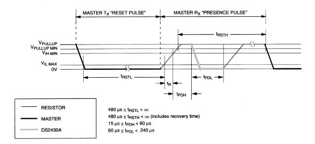
In order not to mask interrupt signaling by other devices on the 1-Wire bus,  $t_{RSTL} + t_R$  should always be less than 960  $\mu$ s.
