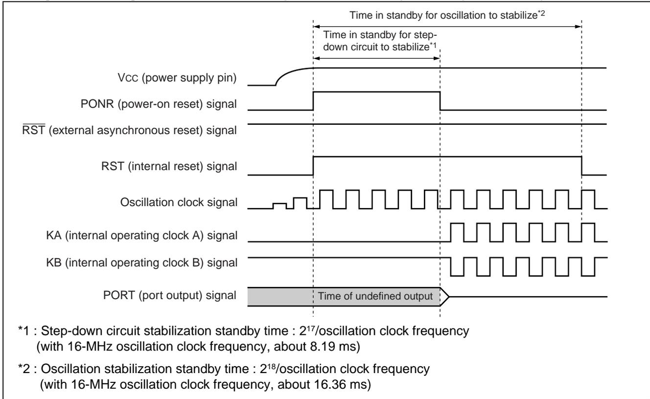
• **Figure 2 - Timing Chart of High Impedance State for Ports 0/1 (when  $\overline{\text{RST}}$  pin is "L")**
