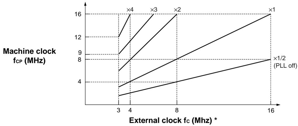
\* : When using the oscillation circuit, the maximum oscillation clock frequency is 5 MHz.
