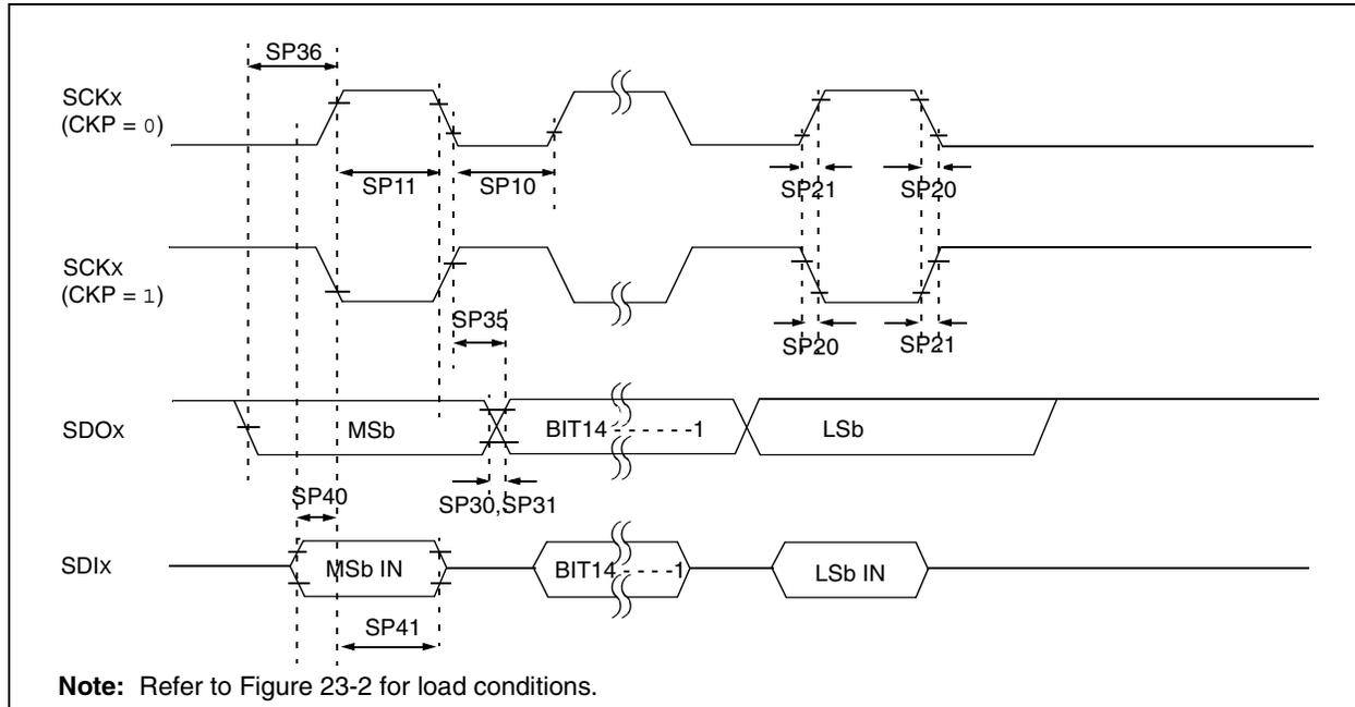
**TABLE 23-33: SPI™ MODULE MASTER MODE (CKE = 1) TIMING REQUIREMENTS**
