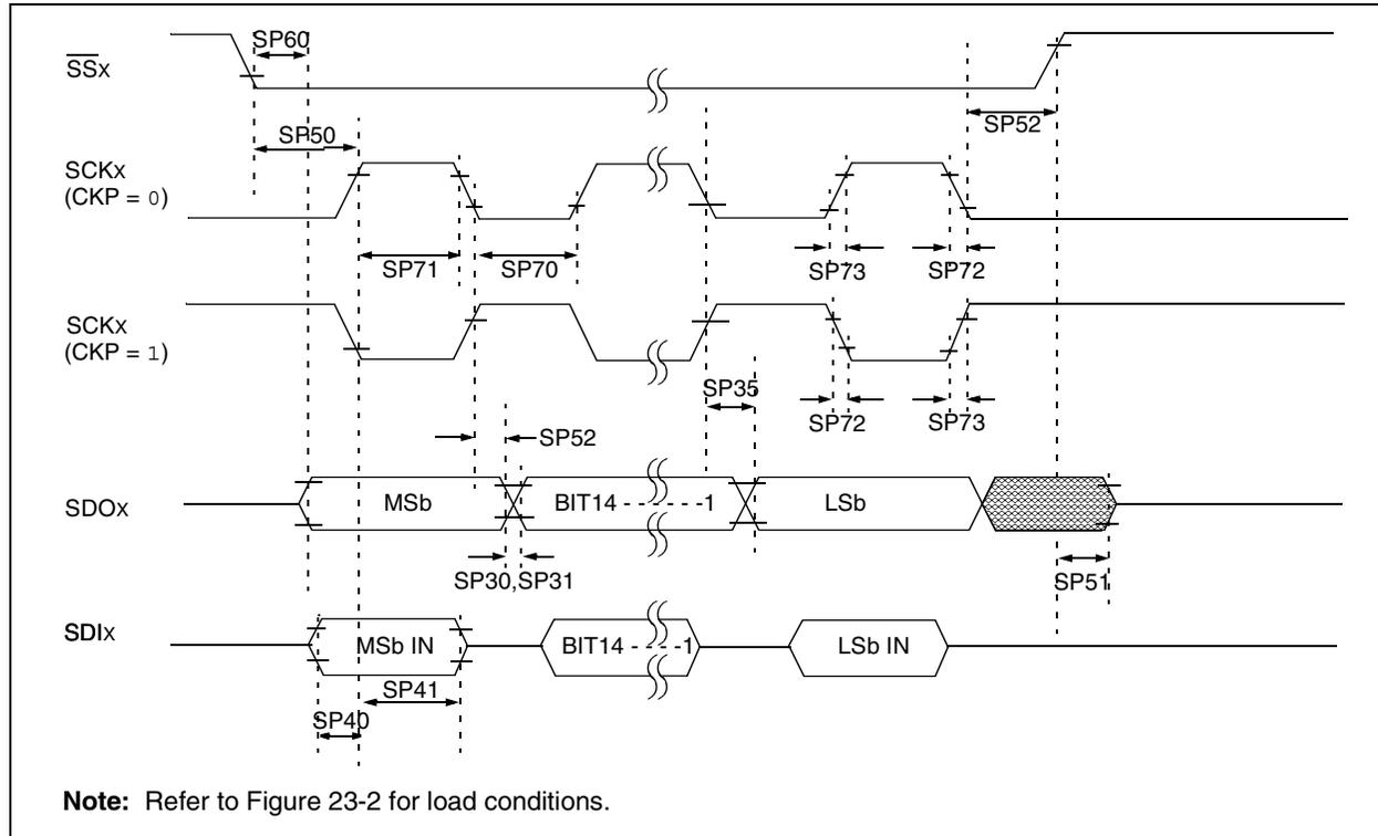
**TABLE 23-35: SPI™ MODULE SLAVE MODE (CKE = 1) TIMING REQUIREMENTS**
