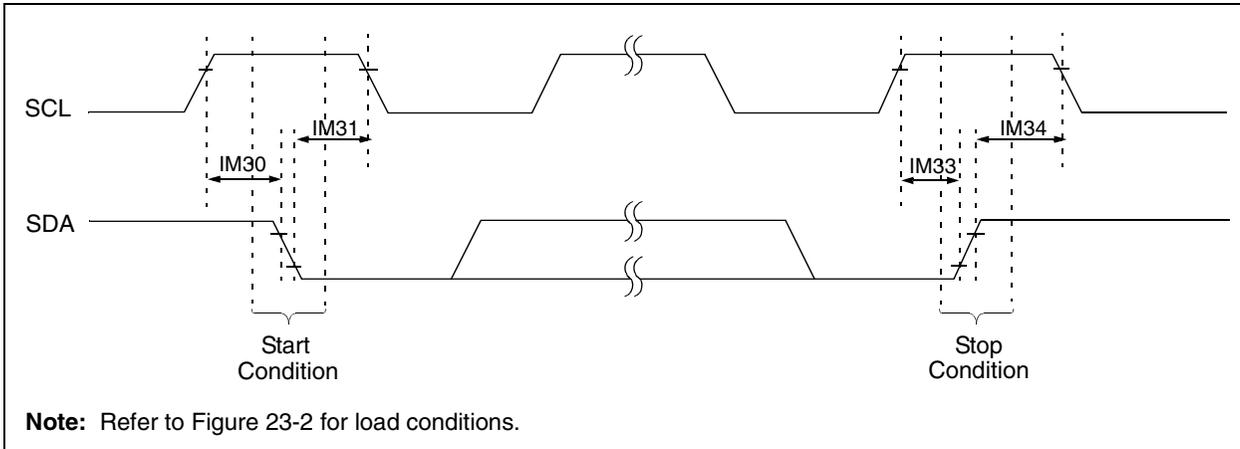
**FIGURE 23-21: I<sup>2</sup>C™ BUS DATA TIMING CHARACTERISTICS (MASTER MODE)**
