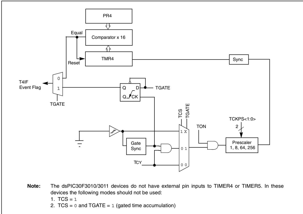
**FIGURE 11-3: 16-BIT TIMER5 BLOCK DIAGRAM (TYPE C TIMER)**
