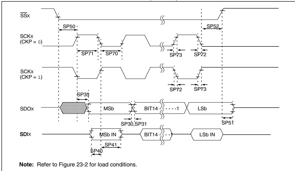
**TABLE 23-34: SPI MODULE SLAVE MODE (CKE = 0) TIMING REQUIREMENTS**
