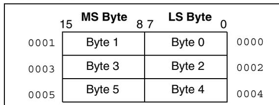
All byte loads into any W register are loaded into the LS Byte. The MSB is not modified.
