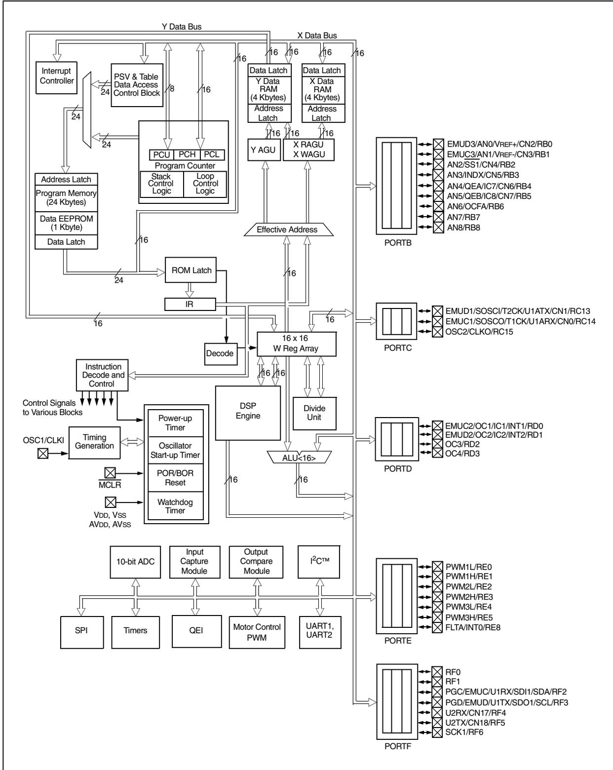
**FIGURE 1-2: dsPIC30F3010 BLOCK DIAGRAM**
