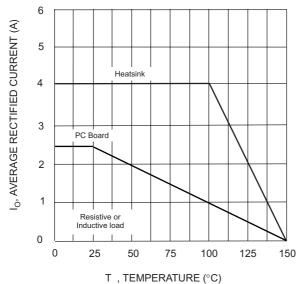
Fig. 1 Forward Current Derating Curve
