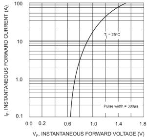
Fig. 2 Typical Fwd Characteristics, per element
