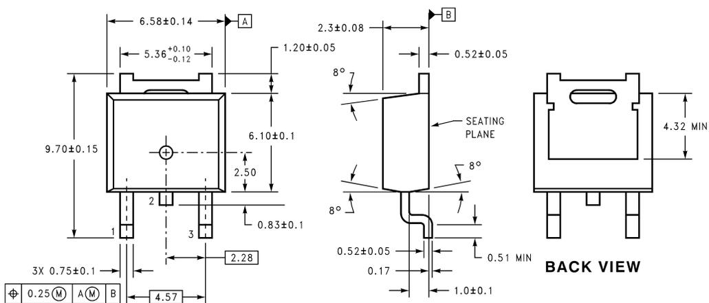
DIMENSIONS ARE IN MILLIMETERS
