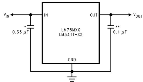
\*Required if regulator input is more than 4 inches from input filter capacitor (or if no input filter capacitor is used).
