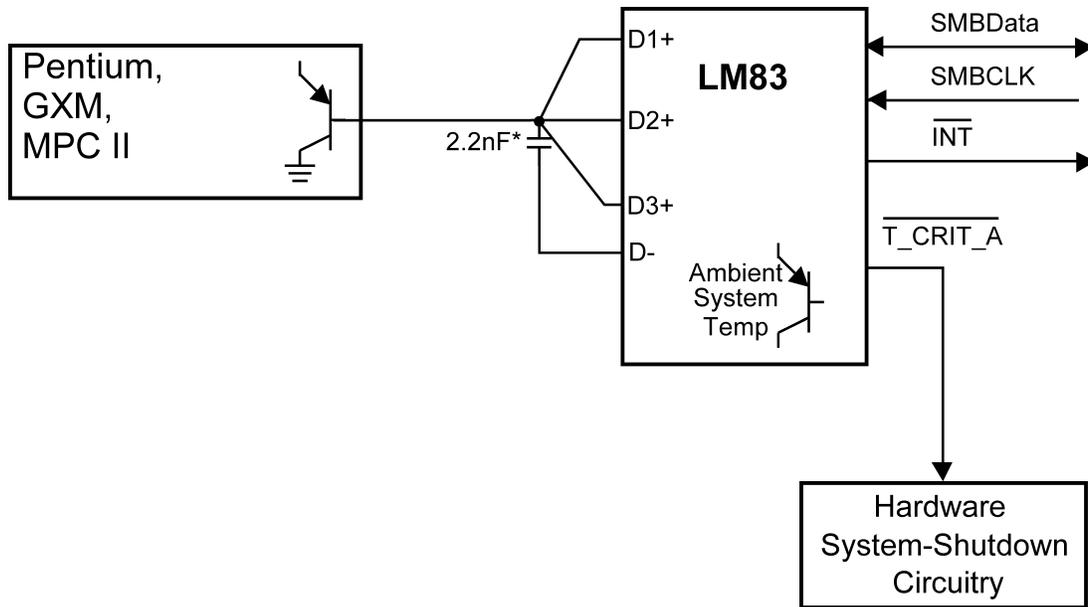
\*Note: 2.2nF Capacitor must be placed as close as possible to D+ and D- pins of the LM83.
