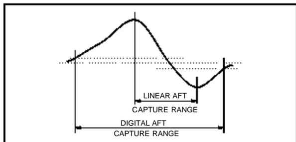
Additionally the use of the Digital AFT allows storage of the tuning information corresponding to the zero point of the AFC-S-curve. This cannot be guaranteed using the Linear AFT method only. The latter is a cheaper system, because it does not require the use of the TDA4433 but it cannot guarantee what described above.
