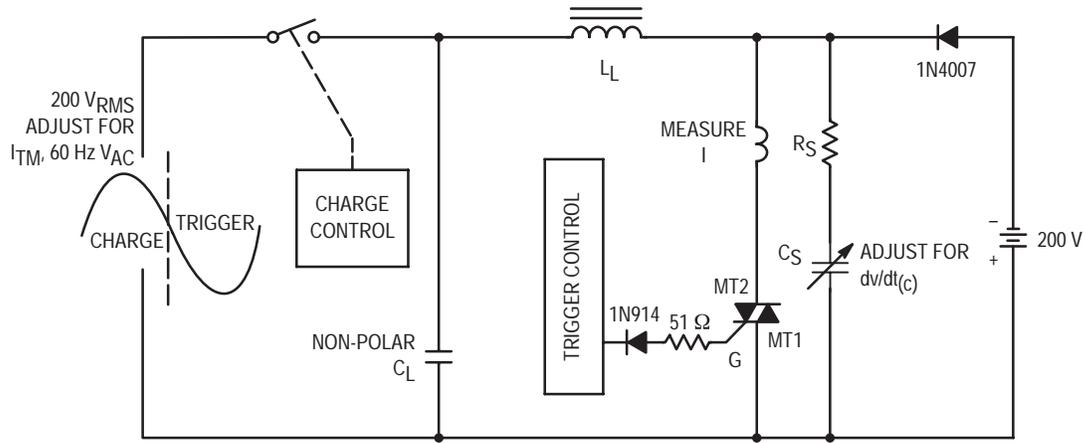
Note: Component values are for verification of rated  $(dv/dt)_c$ . See AN1048 for additional information.
