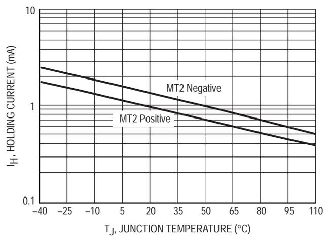
Figure 10. Typical Holding Current versus Junction Temperature
