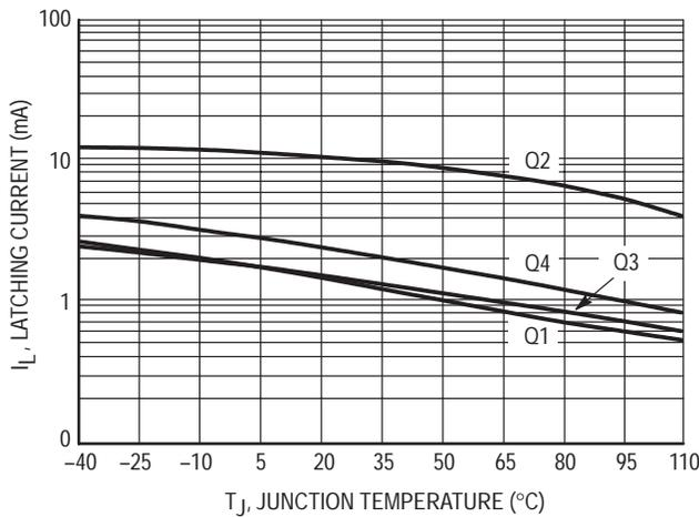
Figure 9. Typical Latching Current versus Junction Temperature
