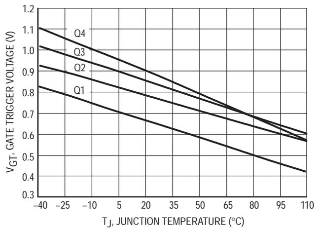
Figure 8. Typical Gate Trigger Voltage versus Junction Temperature
