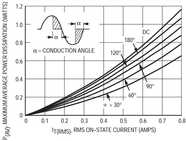
Figure 3. Power Dissipation
