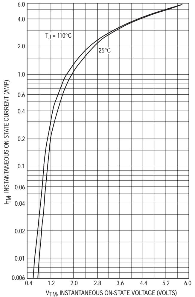
Figure 4. On-State Characteristics
