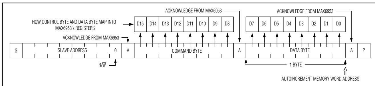
Figure 8. Command and Single Data Byte Received
