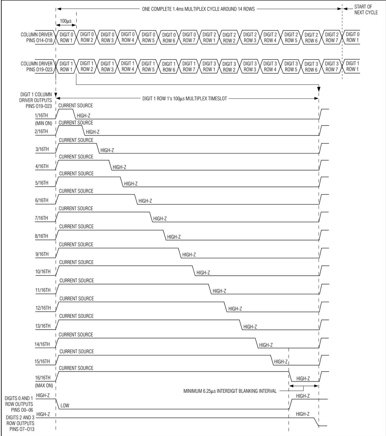
Figure 10. Multiplex Timing Diagram (OSC = 4MHz)
