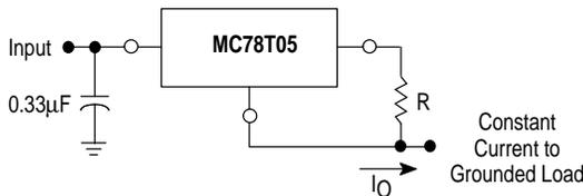
The MC78T05 regulator can also be used as a current source when connected as above. In order to minimize dissipation the MC78T05 is chosen in this application. Resistor R determines the current as follows:
