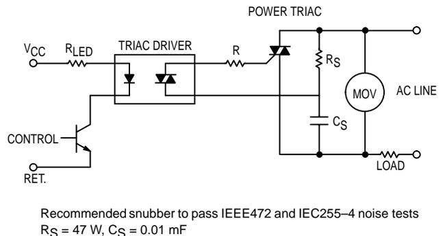
**Figure 13. Triac Driver Circuit for Extremely Noisy Environments**
