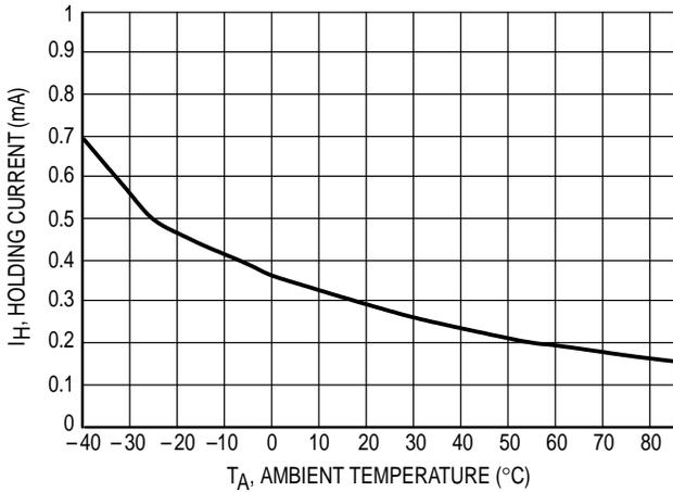
Figure 6. Holding Current, I<sub>H</sub> versus Temperature
