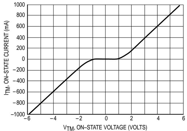
**Figure 2. On-State Characteristics**
