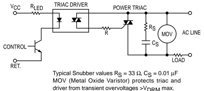
**Figure 12. Triac Driver Circuit for Noisy Environments**
