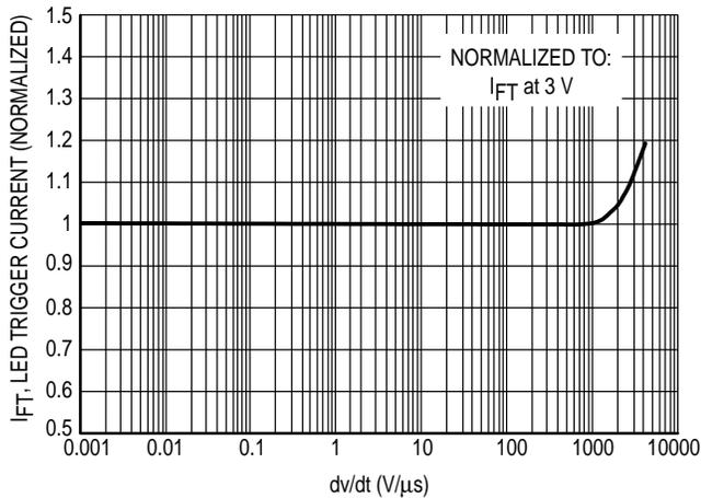
Figure 8. ED Trigger Current, I<sub>FT</sub>, versus dv/dt
