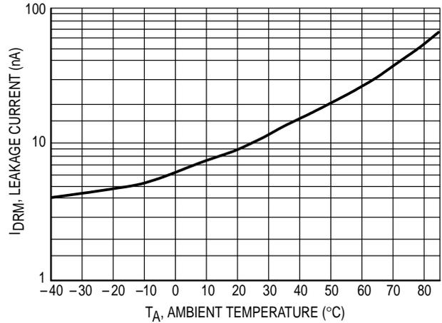
Figure 7. Leakage Current, I<sub>DRM</sub> versus Temperature
