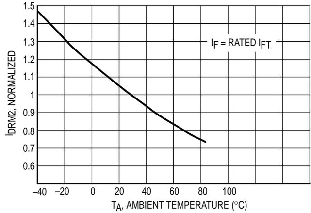
**Figure 4. I<sub>DRM2</sub>, Leakage in Inhibit State versus Temperature**
