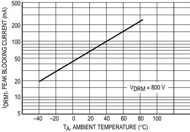
**Figure 3. Leakage with LED Off versus Temperature**
