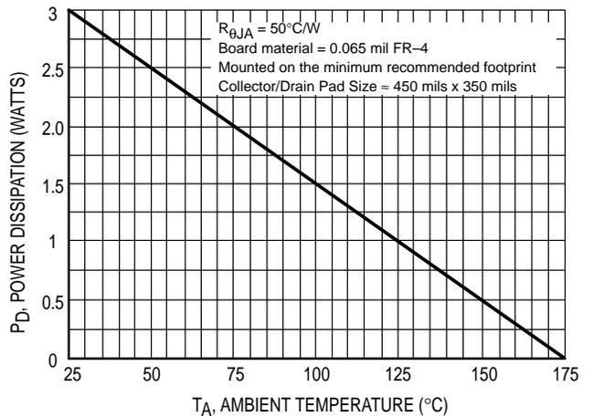
Figure 15. D<sup>2</sup>PAK Power Derating Curve
