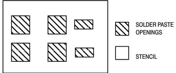
**Figure 17. Typical Stencil for DPAK and D<sup>2</sup>PAK Packages**
