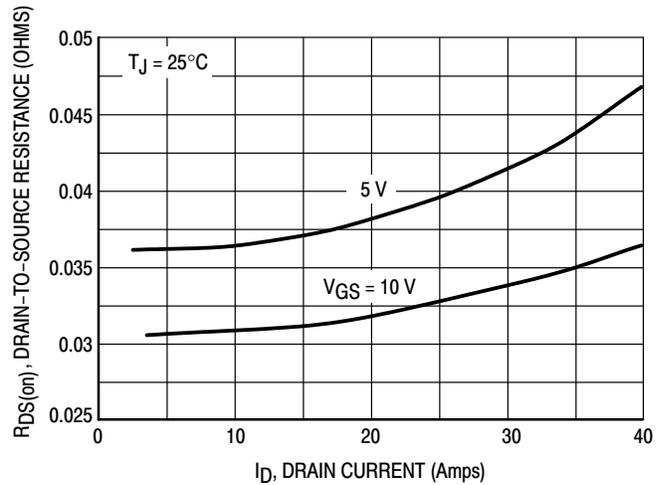
Figure 4. On-Resistance versus Drain Current and Gate Voltage
