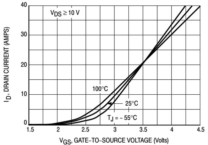
Figure 2. Transfer Characteristics
