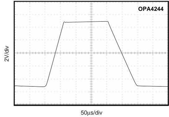
SMALL-SIGNAL STEP RESPONSE,  $G = 1$ ,  $C_L = 100\text{pF}$
