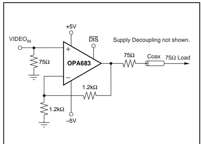
FIGURE 5. Gain of +2 Video Cable Driver.
