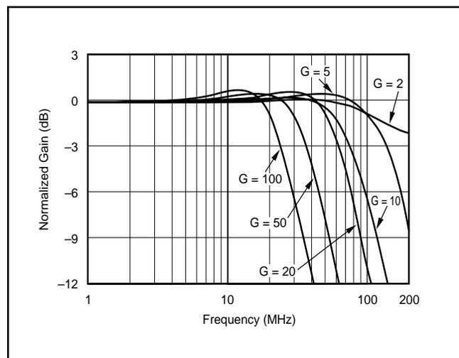
FIGURE 12. Small-Signal Frequency Response with Optimized  $R_F$ .
