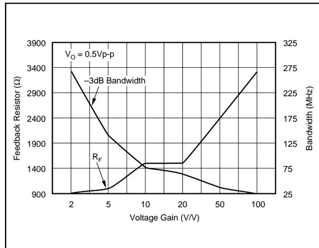
FIGURE 11. Bandwidth and  $R_F$  Optimized vs Gain.
